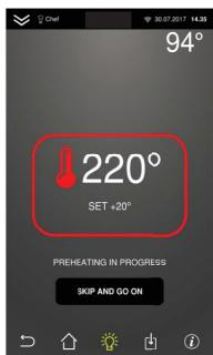
When the preheating reaches the set temperature, the buzzer is activated and the screen on the side is displayed.
