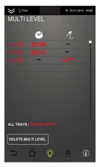
When the time expires, or when the core probe temperature is reached, the buzzer is activated and the number of the tray level to be extracted is shown on the screen.
