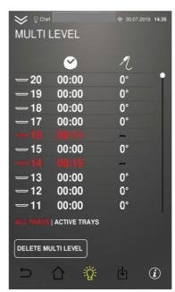
In the operating screen, in the line where the remaining time or the core probe temperature is normally displayed, MULTI LEVEL is displayed to indicate that the cooking duration control is now managed by this function.
